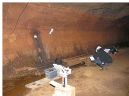
Figure 12: Dr. Rohit Salve setting up an environmental monitoring station on the 4850 Level
